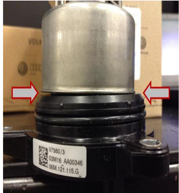
Figure 1. Gap between chamber and seal.
