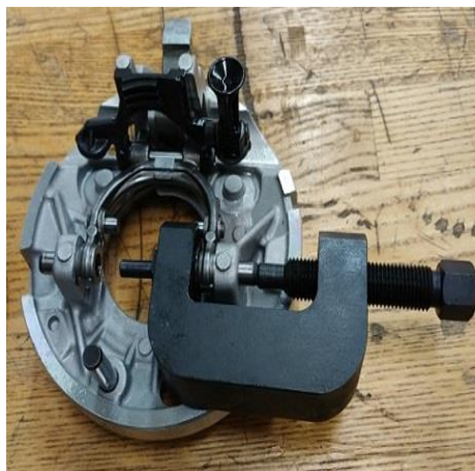
Figure 18. Pin pressing with the 582277.
