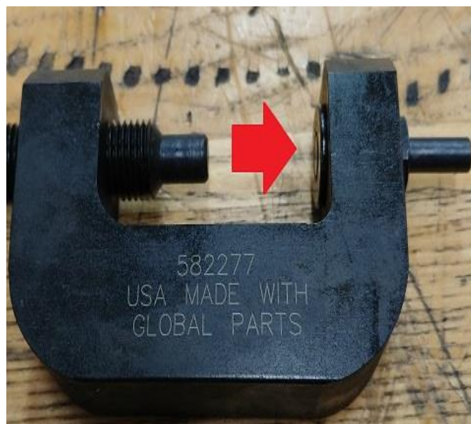
Figure 17. T10172/9 installed in 582277.
