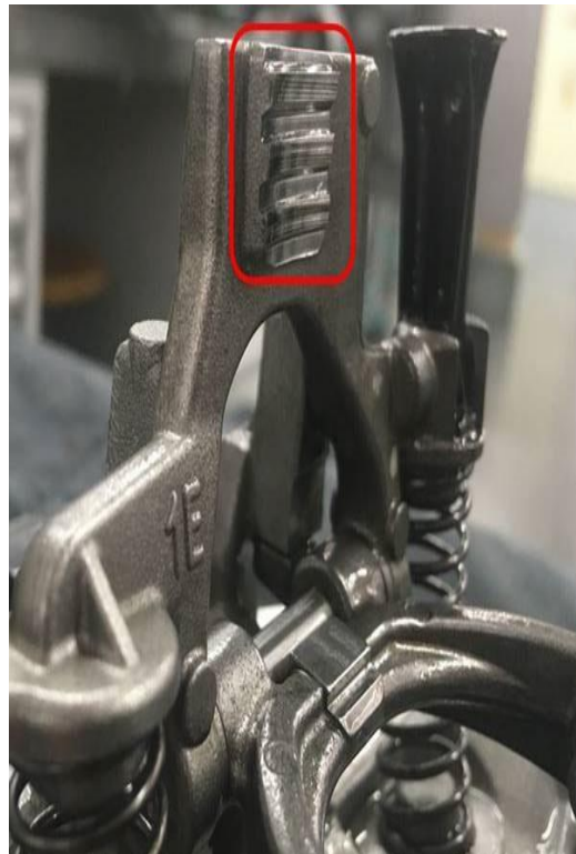
Figure 1. Worn/faulty shift fork.
