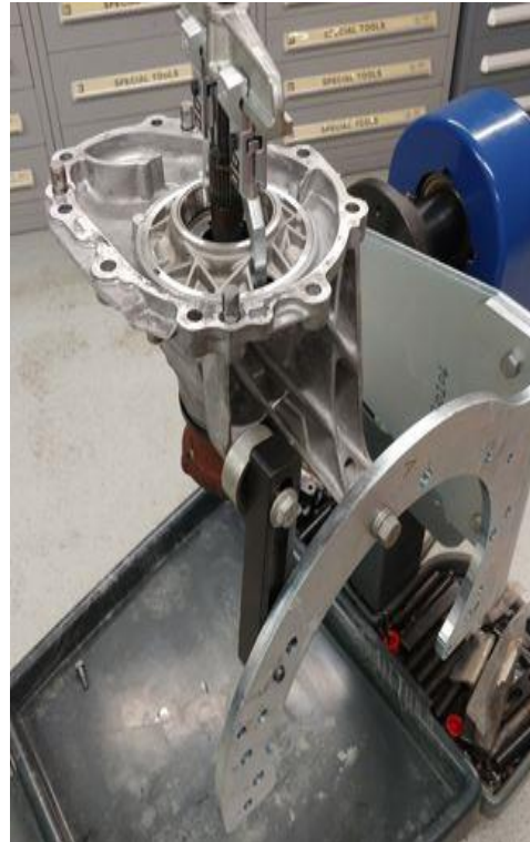
Figure 3. Mounted side carrier.
