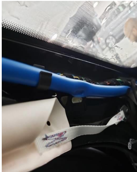
Figure 2. Sunroof drain hose pinched by pillar trim.
