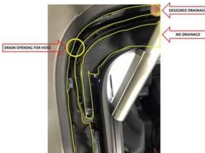
Figure 7. Sunroof water channeling diagram.
