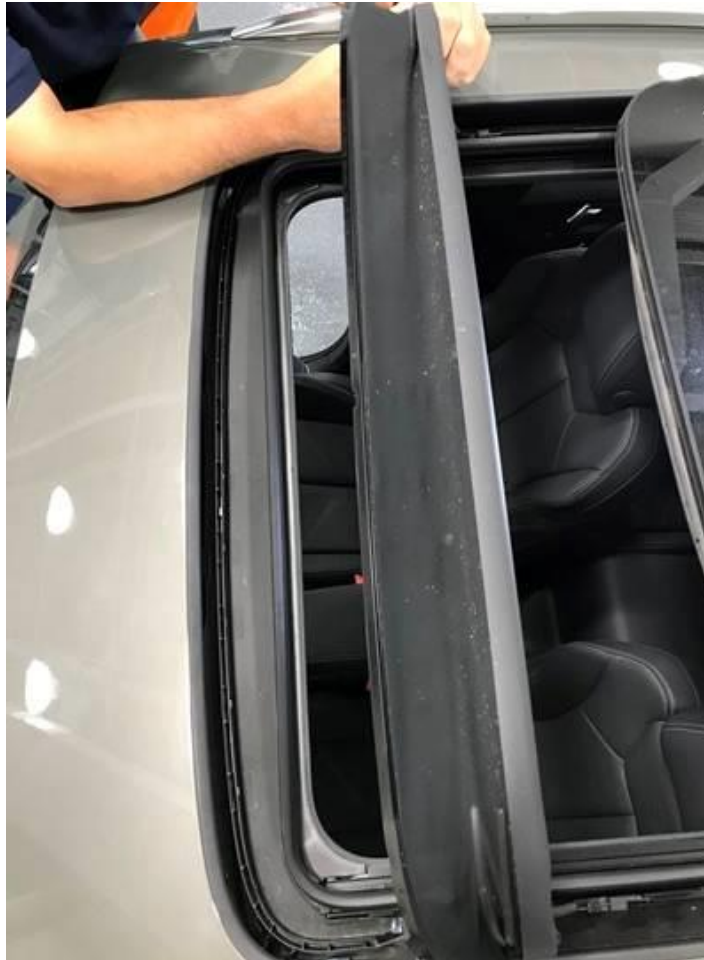
Figure 5. Front sunroof opening with drainage exposed.
