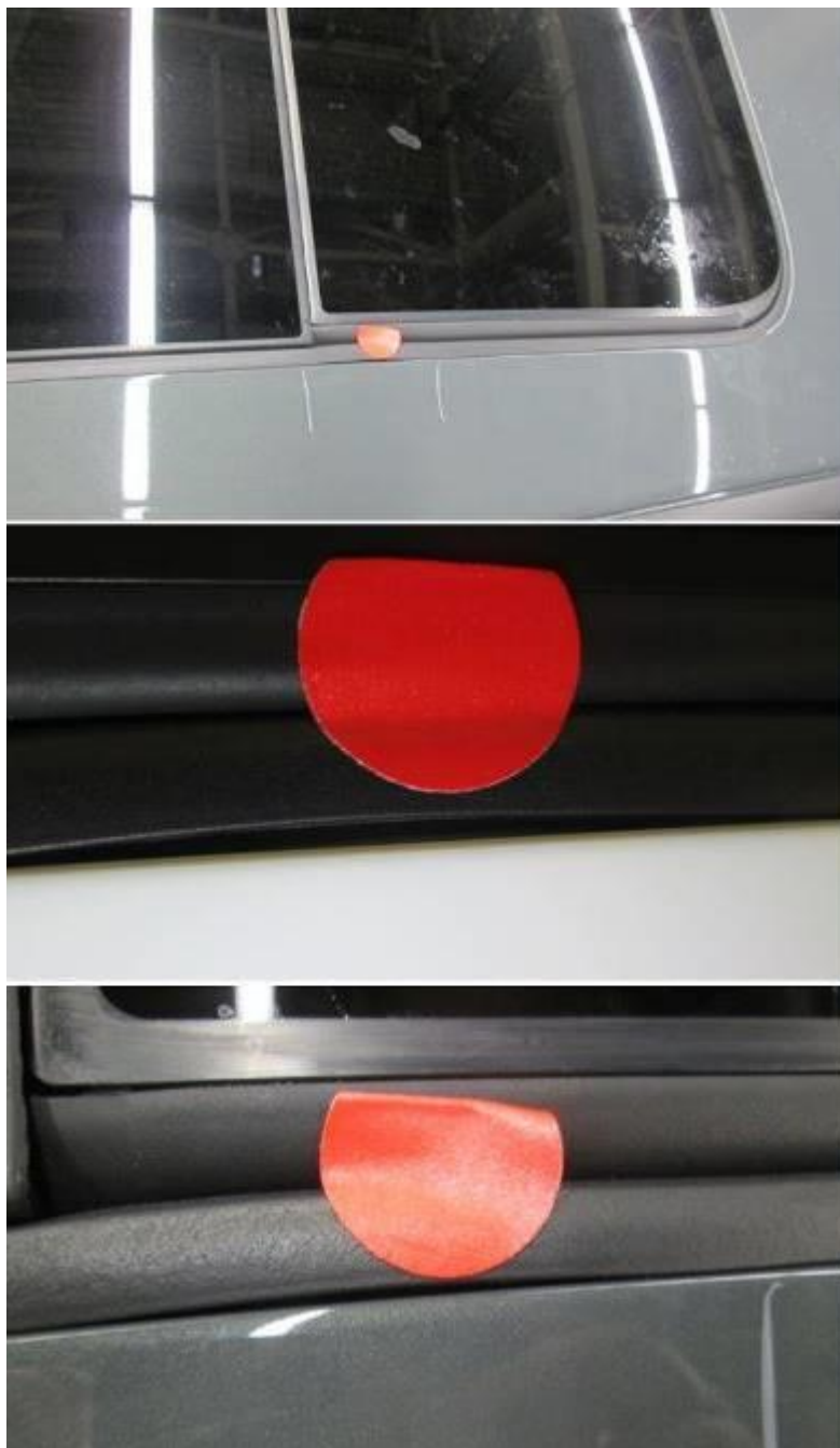
Figure 3. Detached and malformed roof opening seal.
