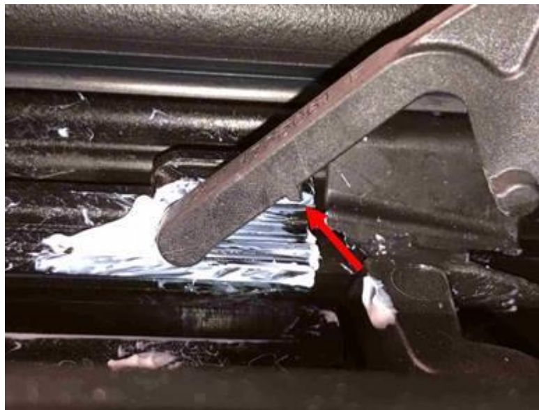
Figure 9. Tabs cast into the redesigned wind deflector.
