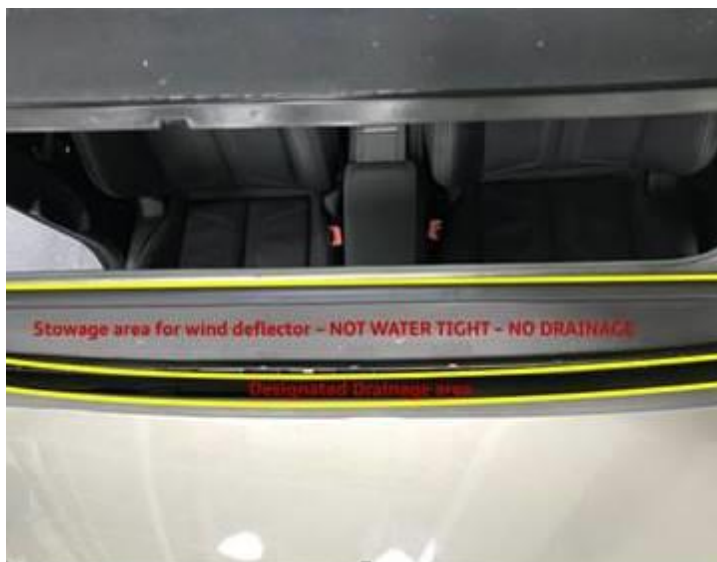
Figure 6. Areas of sunroof opening water elimination capabilities.
