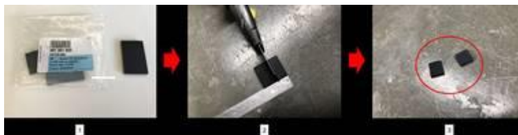
Figure 15. Preparing 2 – 10mm x 10mm pads of 251 201 525 packing.
