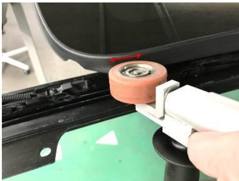
Figure 17. Applying pressure to bonded area with 3356 roller (or equivalent).
