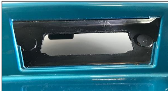
1 Visible Front Area of Steel Reinforcement Panel Painted Black With No Visible Rust
