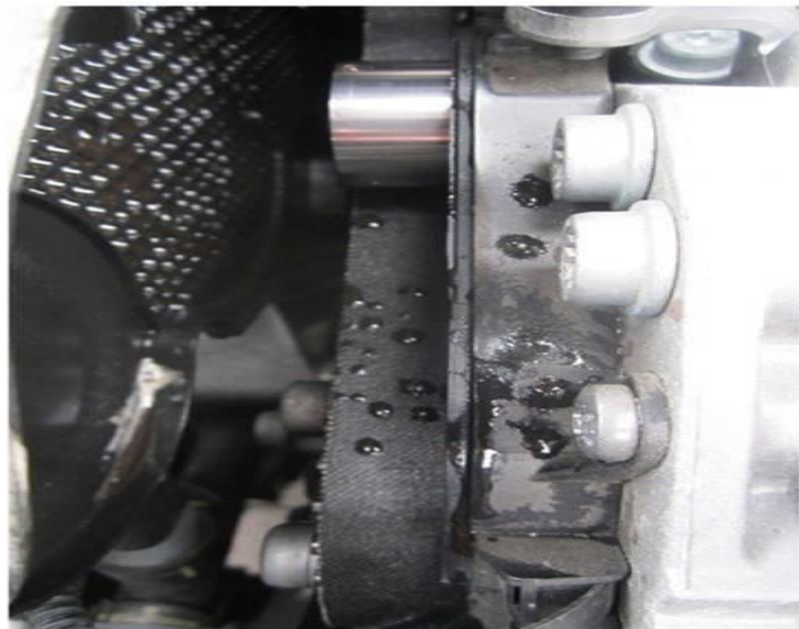
Figure 1. Example of the toothed belt that was briefly in contact with coolant.
