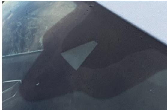
Figure 1. Viewing area fogged up from outside.
