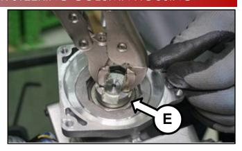
Apply grease to worm gear shaft (E) portion only (OK). Grease should not be applied to the bearing (NG).
