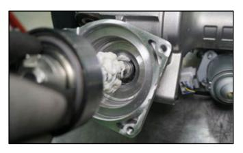
7. Using a torque wrench and SST (B), tighten the shaft nut (C).
