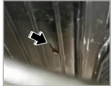
Crack in ATF pan
