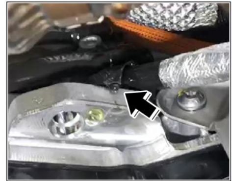
Friction welded joint for ATF cooling line PHEV faulty
