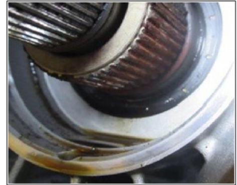
Oil leak on output-shaft sealing ring
