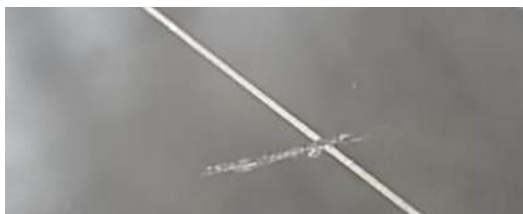
Figure 1. Scratched rear window, visible with the naked eye.
