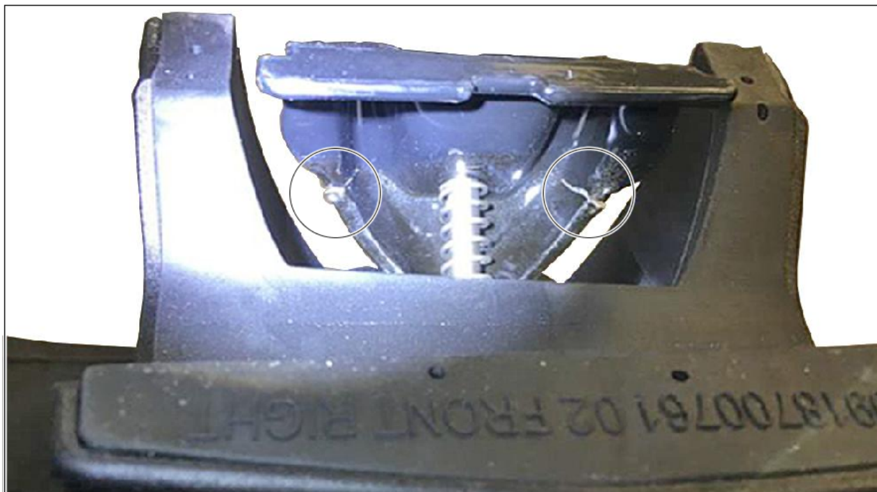
Cracks in clamping plate
