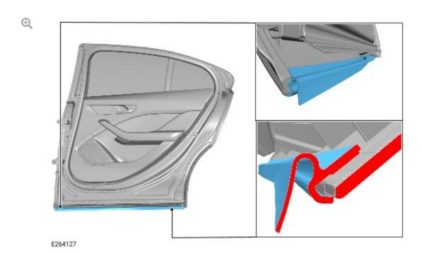
Gradually remove the adhesive backing and install the new rear right door lower seal in small sections at a time. Apply firm pressure along the entire length of the lower seal to make sure the adhesive is bonded to the rear right door lower molding.
