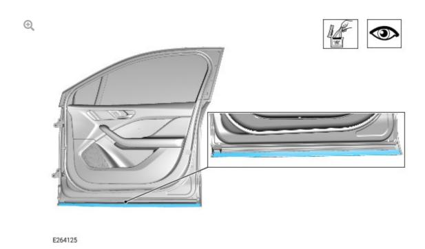
Following the manufactures specifications, apply the  $3M^{\text{\tiny M}}$  adhesion promoter (or equivalent) to the inside edge of the front right door lower molding, as shown highlighted in the illustration.
