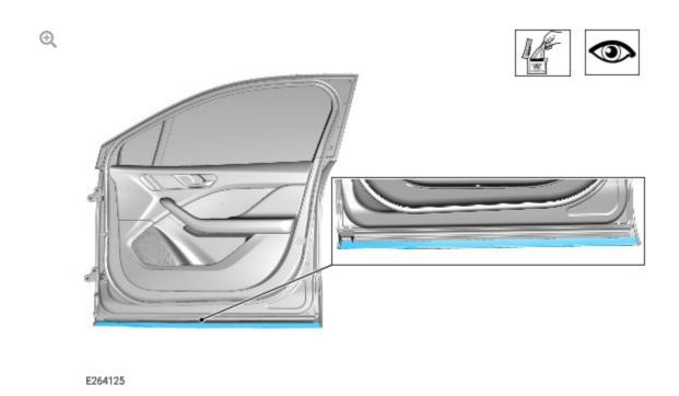
Using 3M<sup>™</sup> surface cleaner (or equivalent), clean the inside edge of the front right door lower molding, as shown highlighted in the illustration.
