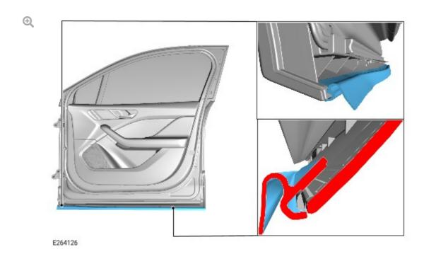
Gradually remove the adhesive backing and install the new front right door lower seal in small sections at a time. Apply firm pressure along the entire length of the lower seal to make sure the adhesive is bonded to the front right door lower molding.
