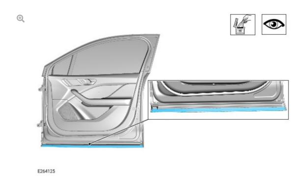
Following the manufactures specifications, apply the  $3M^{\text{\tiny M}}$  adhesion promoter (or equivalent) to the inside edge of the rear right door lower molding, as shown highlighted in the illustration.
