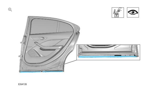
Using 3M™ surface cleaner (or equivalent), clean the inside edge of the rear right door lower molding, as shown highlighted in the illustration.
