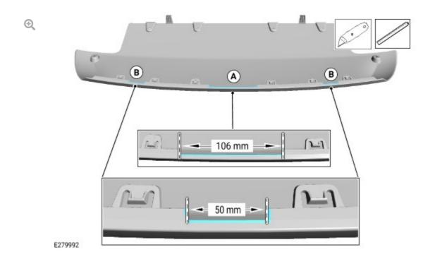
Using a suitable tool, modify the front towing eye cover, as shown in the illustration. Make sure an equal amount of material is removed from each side of the slotted area, which will allow the slotted area to remain central, between the fixing tabs.
