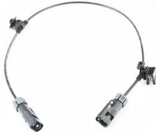
Figure 1. 69Z4 campaign harness obsolete after PODS Repair Kit installation.
