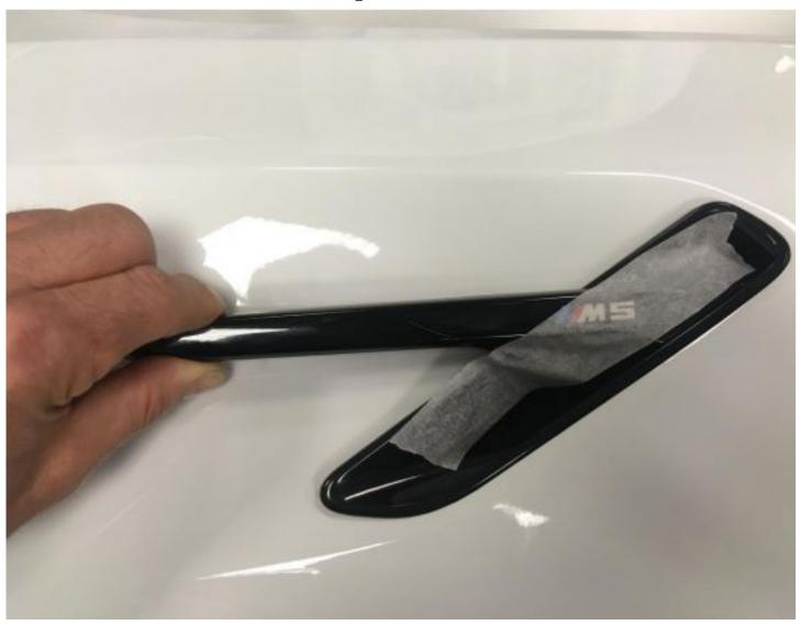
6. After 3 hours, the adhesive tape can be removed. Allow 24 hours of curing time before washing the vehicle.
