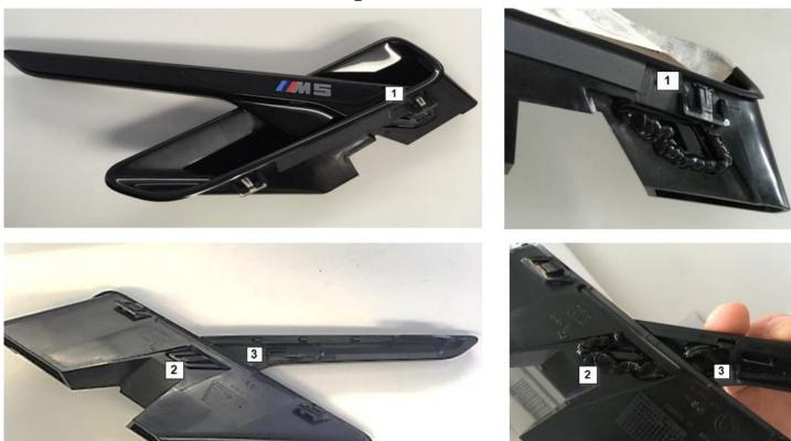
Note: The adhesive at position 3 will be used to bond the air duct cover to the fender. See step 4 for additional instructions for this position.
