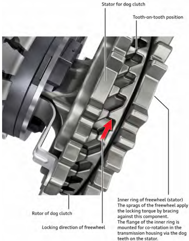
Dog clutch aligned tooth on tooth
