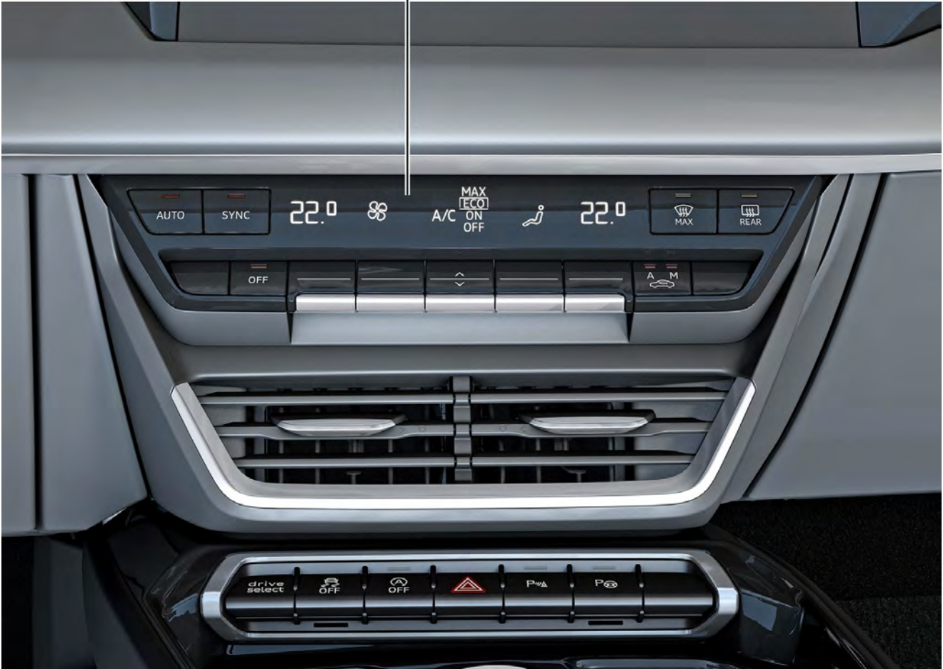
Operating and display unit for front air conditioning system E87
