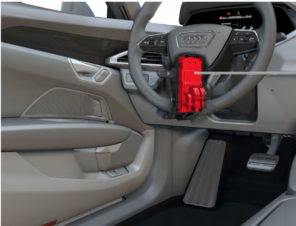
Onboard supply control unit J519
