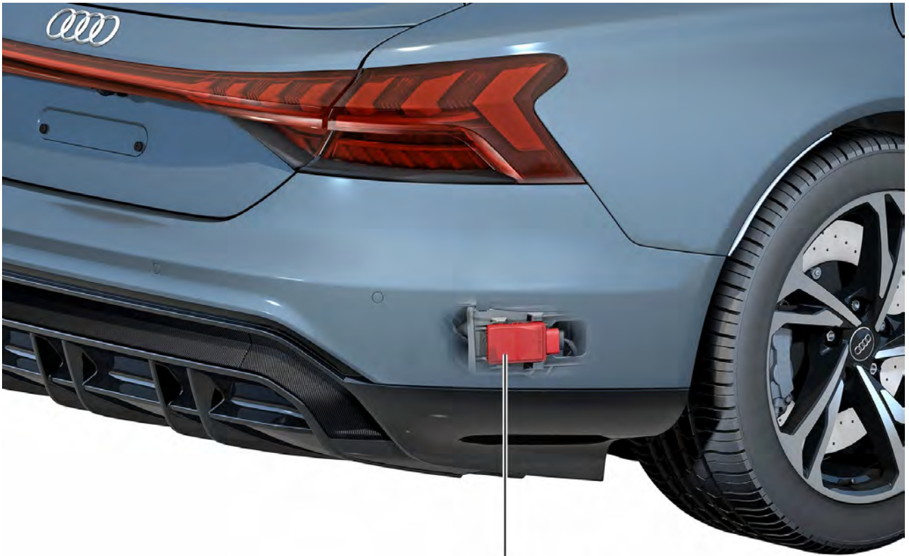
Right rear radar sensor (lane change assist control unit 2 J770)
