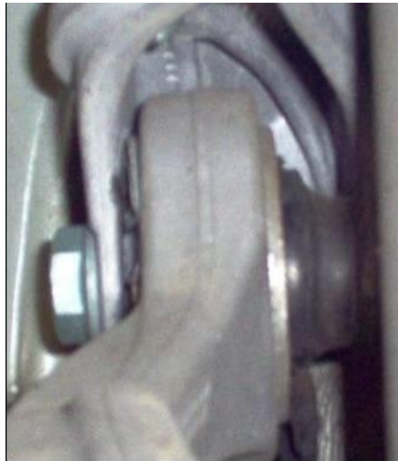
Figure 4. A bushing with a displaced insert, shown installed in the vehicle.
