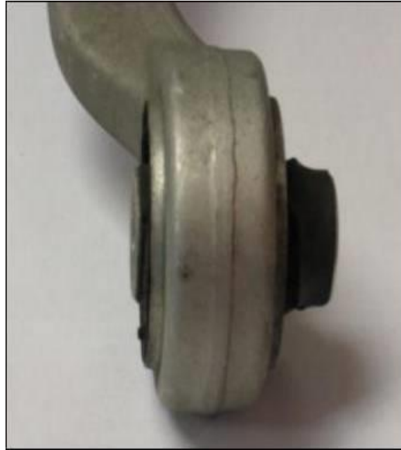
Figure 3. A bushing with a displaced insert.
