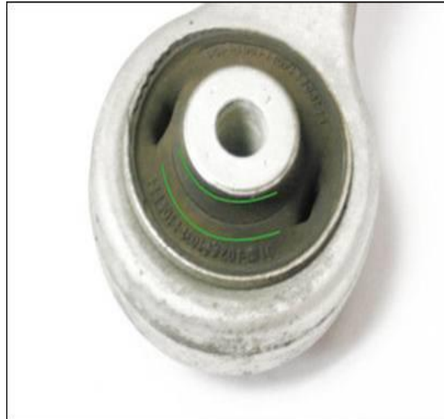
Figure 5. A bushing with a hairline crack. This is an acceptable amount of wear.
