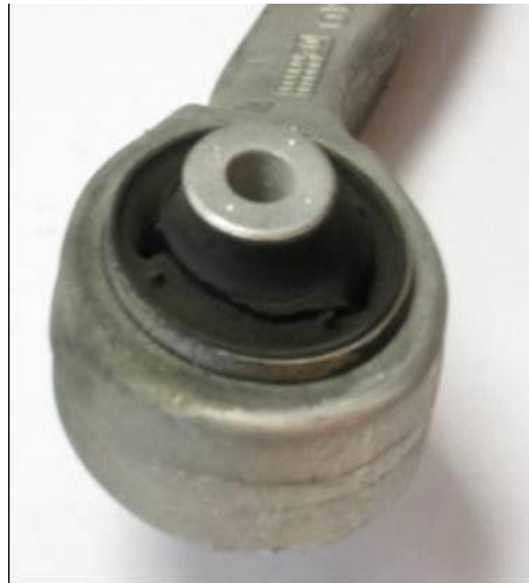
Figure 2. A bushing with cracked rubber.
