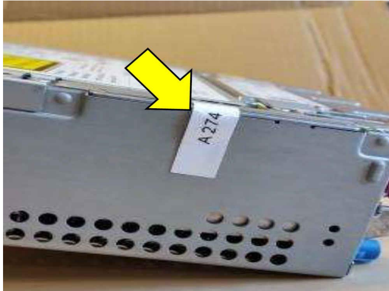
Figure 9. Place the new warranty seal over the location indicated by the yellow arrow.
