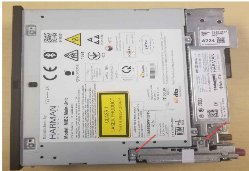
Figure 6. Telephone module retaining screws indicated by the red arrow.
