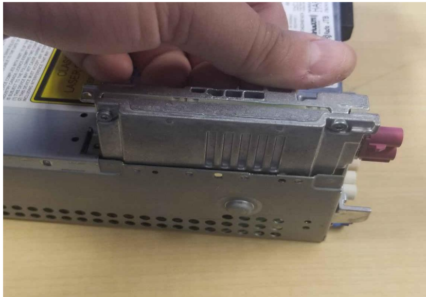
Figure 8. Do not press down using the purple FAKRA connector.
