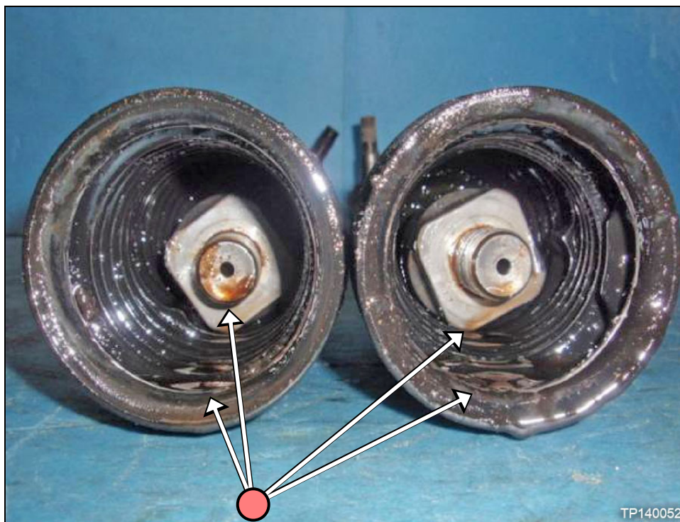
Figure 11: If fluid is red in color, the steering rack is leaking.
