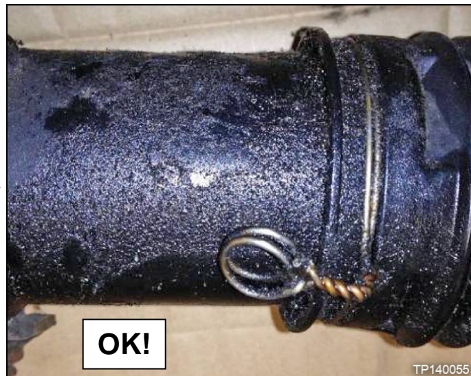
Figure 14. Yes, the steering rack above is OK (not leaking power steering fluid). The extra greasy appearance was caused by an excessive amount of assembly lube.
