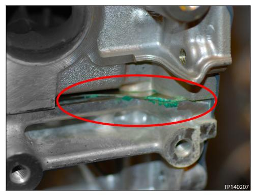
Pictures of acceptable coolant seepage (crusting)
