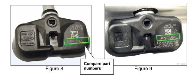
To confirm the latest part numbers, always consult the appropriate parts catalog when replacing or exchanging TPMS sensors, receivers, or control modules.
