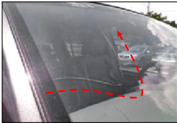
Single crack with no impact mark: Warranty
