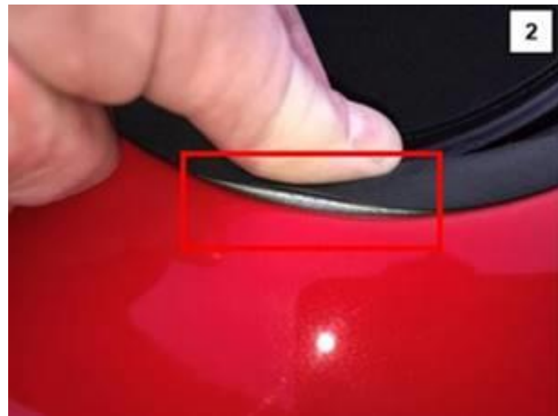
Figure 2. Checking the adhesion quality.
