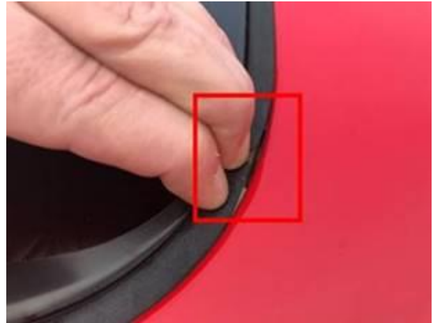
Figure 7. Adhesive band detachment.
