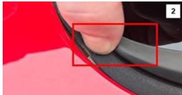
Figure 5. Clear evidence of adhesive detachment.
