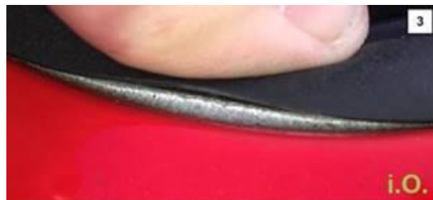
Figure 3. A properly adhered perimeter seal.
