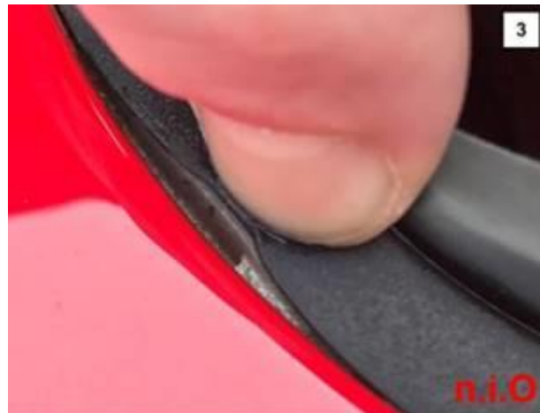
Figure 6. Seal adhesive band detachment revealed.
