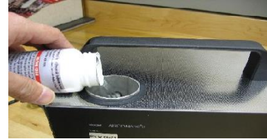
Figure 2. Pouring the treatment into the filling chamber.
