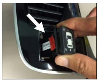
Reinstall switch and verify proper operation. Verify switch is secured by the 2 locking tabs.
