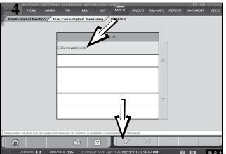
17. Verify the thumb drive is highlighted and touch the **check mark** to continue.
