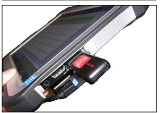
14. To save a permanent record of the Drive Recording, insert a thumb drive into the side USB port.
