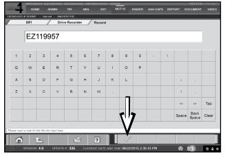
9. Change the name of the file using the last 8 digits of the VIN to identify the file (for example: EZ119957 Drive Record).
