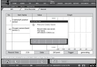
13. After the recording has ended, this screen appears to confirm the recording was saved to the ToughPad<sup>®</sup>.
