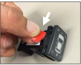
**Repair Procedure:** Remove the Park Assist switch from the panel. Add a 3M tape or equivalent onto the left side of switch (as shown above). Dimensions: L 20mm x W 10mm and thickness of 1.5mm
