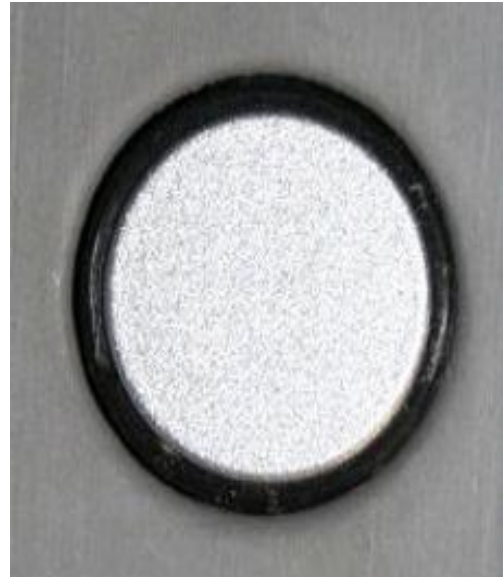
Figure 5. A correctly seated decoupling ring.
