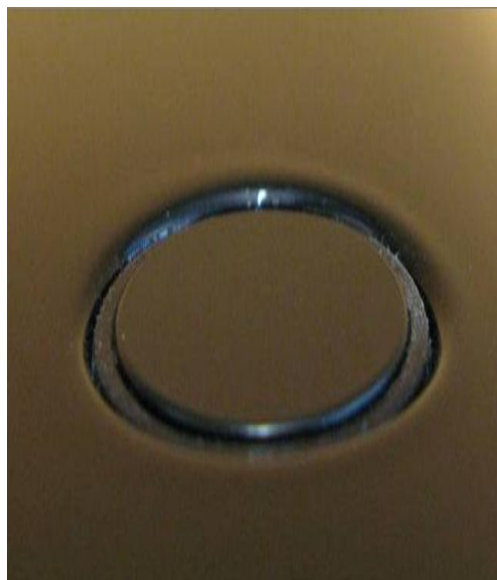
Figure 10. A correctly installed parking aid sensor.
