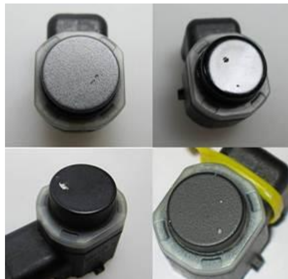
Figure 3. Stone chips causing sensor failure.
