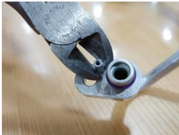
Figure 15. Removal of dowel pin.
