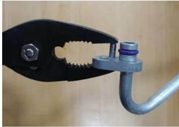
Figure 16. Installation of rear refrigerant line dowel pin.
