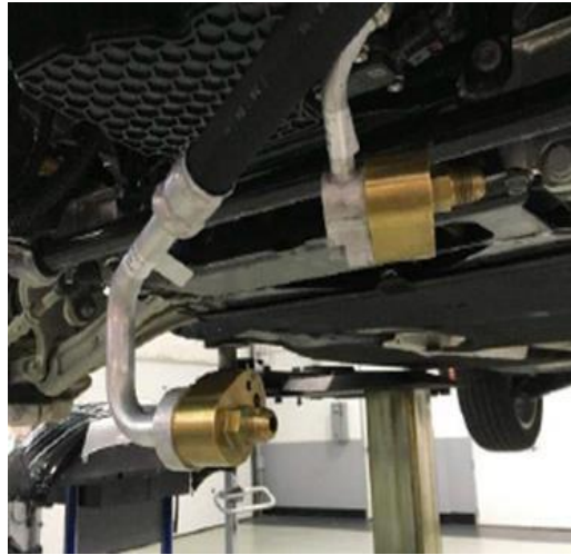
Figure 6. Installation of VAS 6338/3 and 6338/12.
