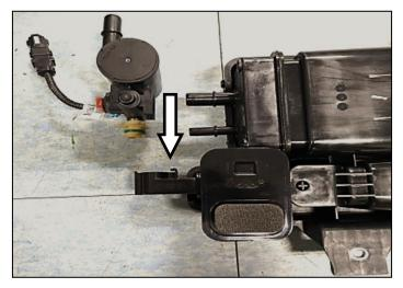
10. Insert the air hose length of 10mm over fresh air and install the other end over the air filter nipple.
