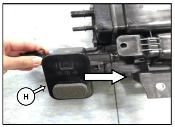
7. After full insertion, rotate 45 degrees counterclockwise to fully seated at the upright position.
