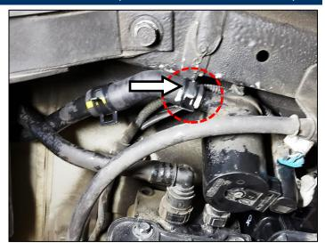
11. Reconnect the CCV wiring connector.
