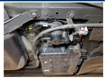
Install the CCV and the air filter assembly to the auxiliary canister.
