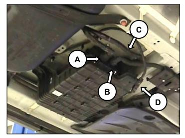
2. Remove the canister protector installation bolts & nut.
