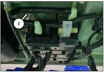
Cut the fresh air ventilation tube ( I ) that connects to the air filter by 180mm.
