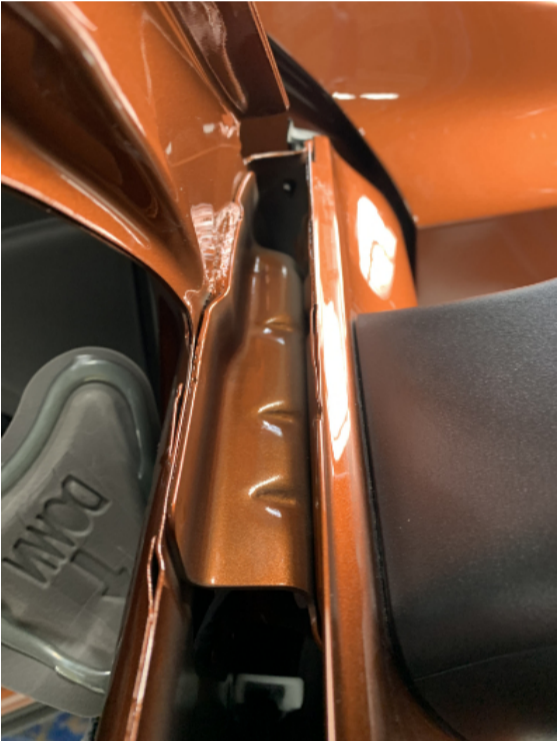
Void where Stuffer will go with Front Side Door Window Weather strip removed
