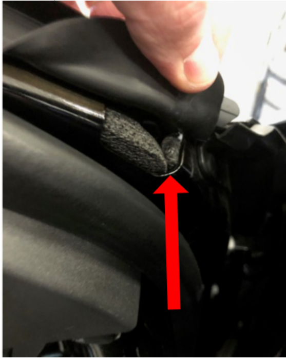
Seal out of position (Note how it sits lower)
