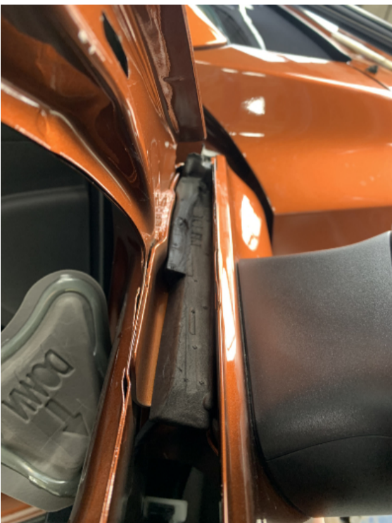
Proper Stuffer orientation in the channel
