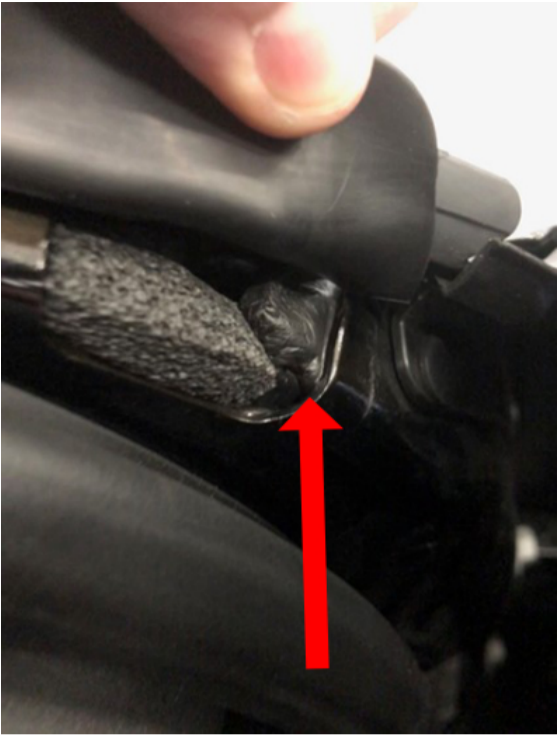
Seal out of position (Note how it sits lower)
