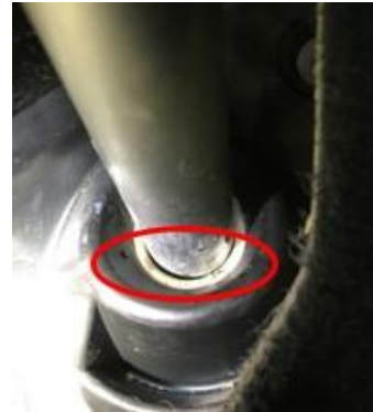
Figure 1. Poor sealing on the intermediate shaft.
