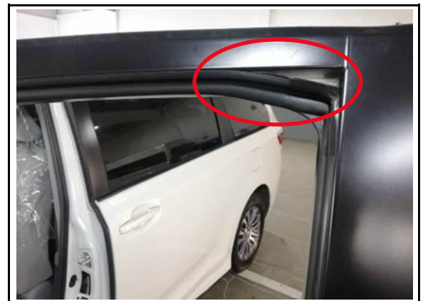
Figure 1. Front Door Glass Run Failure
