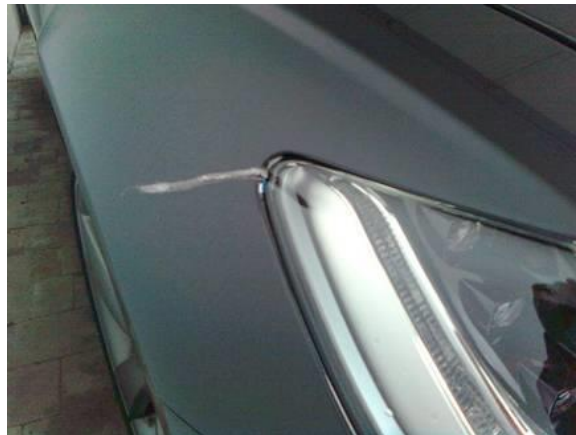
Figure 1. Car wash bristle is stuck in the body gap.
