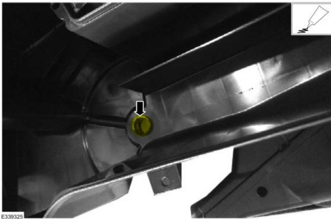
Figure 7 - Arrow indicates where to lubricate the climate control housing surface for the temperature blend door
