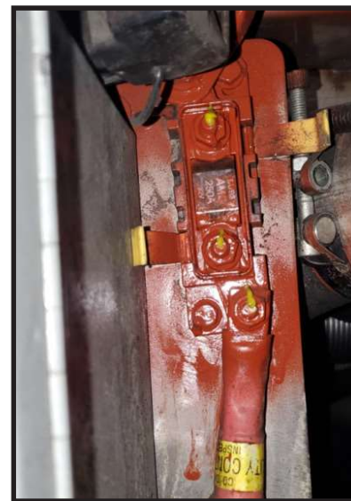
Figure 12 - Dolph ER-44 and Yellow Torque Seal Applied
