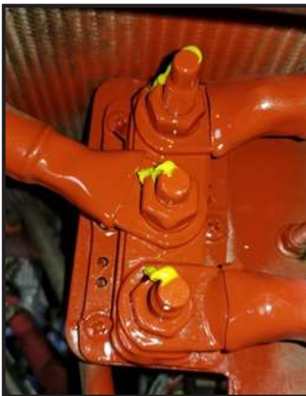
Figure 12 - Dolph ER-44 and Yellow Torque Seal Applied
