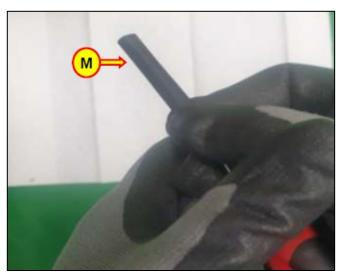
15. Remove the burr while rotating in the circular direction as shown by the arrow for about 8 ~ 9 times while maintaining a perpendicular angle to the WTS mounting hole.
