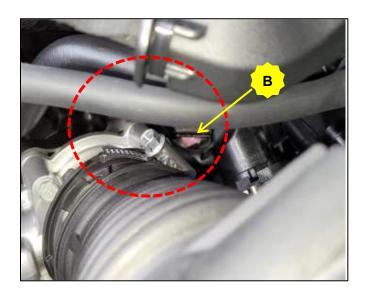
Inspect for coolant leak residue near the cylinder head gasket (A), and areas near the lower end of the intake hose and the intake manifold (B).
