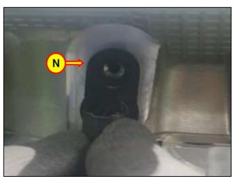
17. To complete the WTS installation, check that the O-ring is fully seated into the mounting hole and then fasten the mounting bolt while initially holding the WTS flat against the cylinder head.
