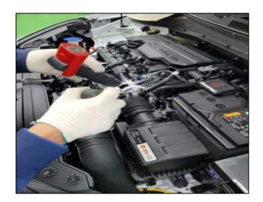
The area to be inspected for coolant leak is the cylinder head and surrounding portions near the mid-point between the intake manifold and intake hose.
