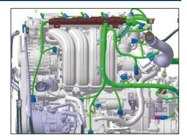
11. Loosen the intake manifold fixing nuts & bolts and remove the intake manifold.
