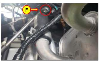
Only loosen the upper mounting bolt (F).
