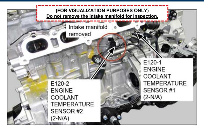
As shown above at areas surrounding sensor #2, visually check for signs of coolant leak.
