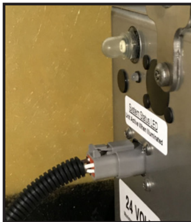
Figure 5 - View of the Super Capacitor Control Connector to Disconnect
