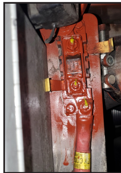
Figure 12 - Dolph ER-44 and Yellow Torque Seal Applied
