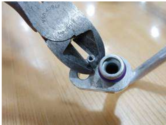
Figure 15. Removal of dowel pin.
