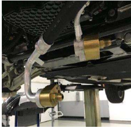
Figure 6. Installation of VAS 6338/3 and 6338/12.
