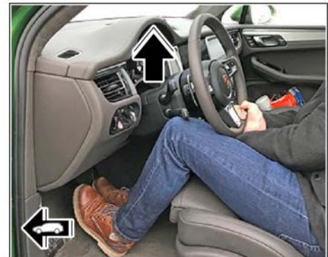
Electric steering column (shown on Macan)
