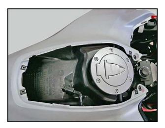
11. <u>In order to improve the coupling of the fuel tank fill cap cover with the fill cap itself and/or the closure of the mobile phone compartment, it is necessary to work on the 6 lateral screws (7), right and left, and on the 2 upper screws (5) fixing the tank fairing (8).</u>
