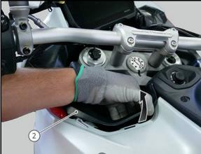
3. Remove the **RH side fairing (2)** (see Sec. 5: "Fairing installation – Tail guard and side body panels" of the Workshop Manual). Follow the same procedure for the LH fairing.
