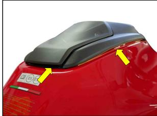
It is possible to realign the Fuel Tank's Fill Cap Cover and the Mobile Phone Compartment Cover by acting on the fuel tank cover fixing screws. In cases where, after following the operations described below, it is not possible to restore the alignment to an acceptable value (for example due to the deformed cover), fill out a **YouTech** service request. Be sure to include notes describing your actions and the issue, as well as clear photos of the alignment problem.
