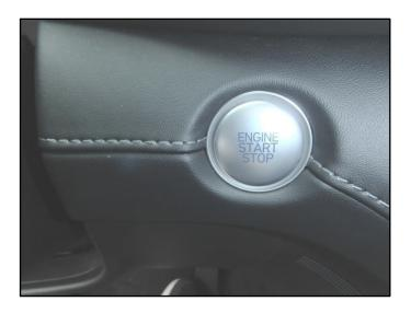
2. Using a plastic pry tool, begin the removal at the indicated position where a slot is located for inserting a removal tool.
