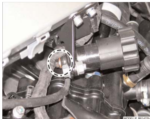
Figure 2: tight spot at banjo bolt
