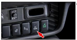
a. To enable power to the 120V AC outlets on the Outlander PHEV, press the "AC 1500W" switch in the front instrument panel (below the A/C controls).
