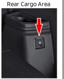
Verify the outlet(s) function properly when an electrical appliance (e.g., coffee maker, blender, etc.) is connected.
