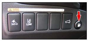
Push the fuel door release button on the lower dash left of the steering wheel.
