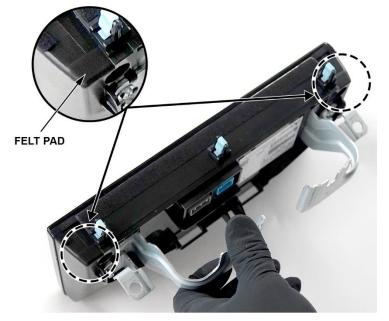
NOTE: Make sure the felt is not visible after screen installation.
