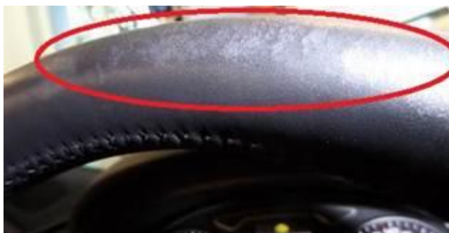
Figure 3. Example of damage from external impact.
