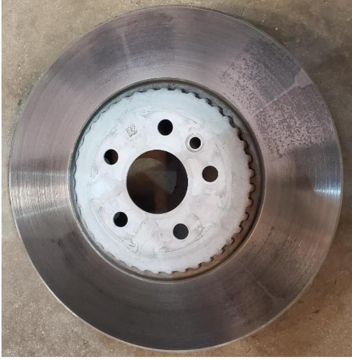
Examples of uneven brake pad material transfer onto the brake disc.
