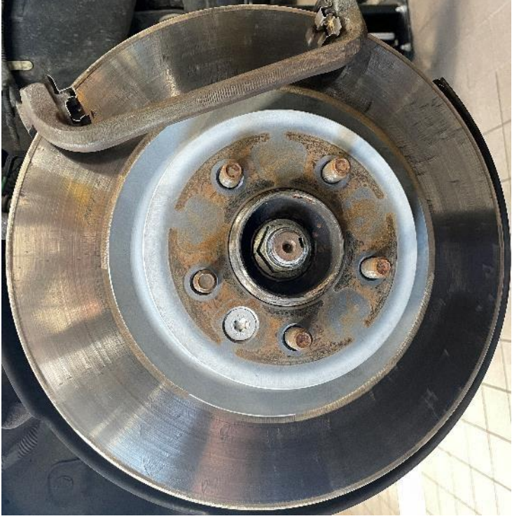
Examples of brake discs improperly sanded with a rotary tool causing a noise concern.
