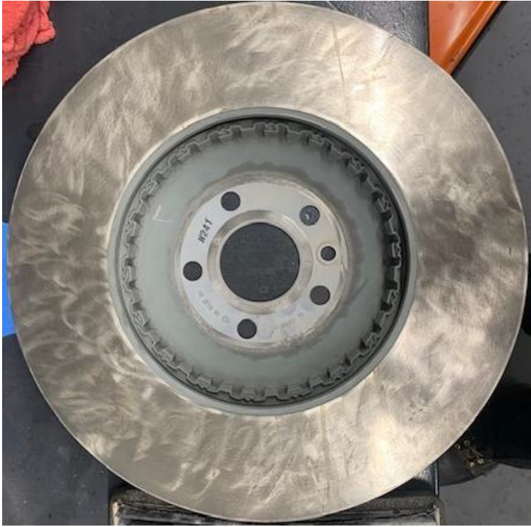
Examples of brake discs improperly sanded with a rotary tool causing a noise concern.
