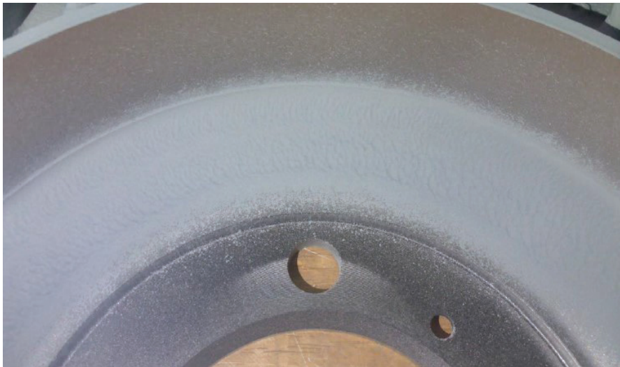
Figure 2: Painted inner surface of brake bell
