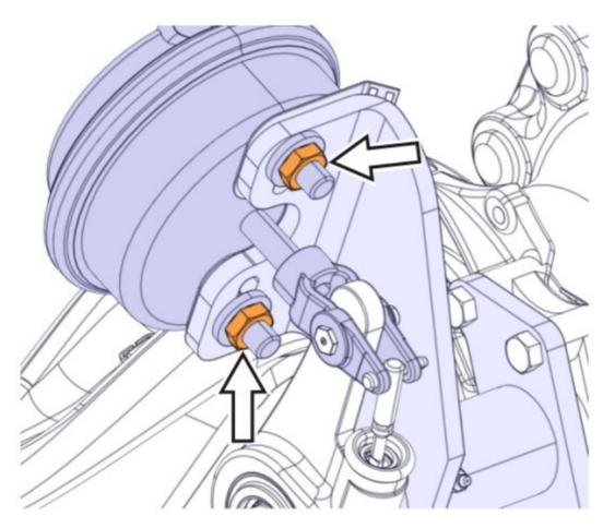
. For Haldex slack adjusters, install the fasteners securing the slack adjuster to the cam tube bracket. . Tighten the slack mounting strap fastener to 11 – 16 Nm (8 – 12 ft-lb).
