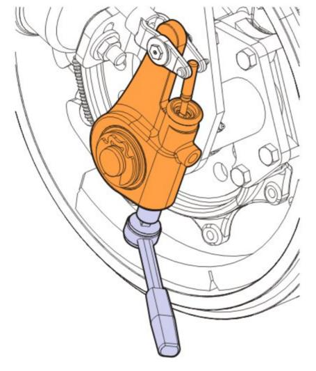
. Remove the brake drum.
