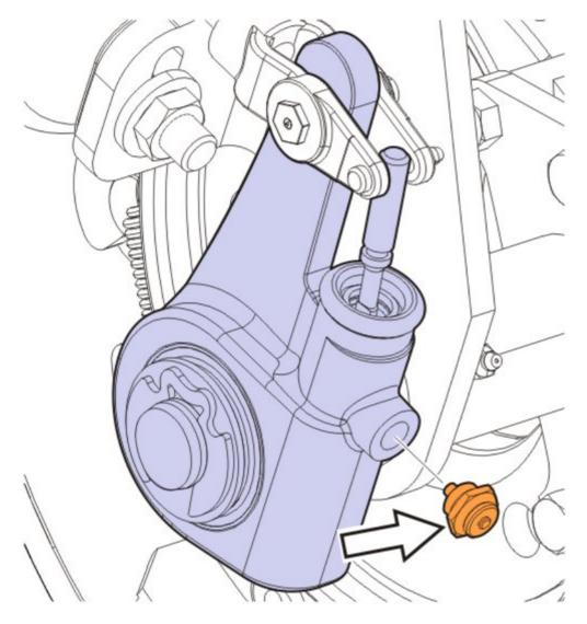
. Back off of the brake (slack adjuster).
