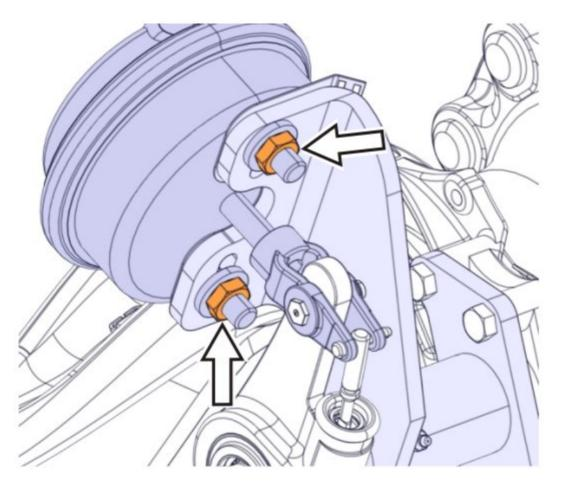
. For Haldex slack adjusters, remove the fasteners securing the slack adjuster to the cam tube mounting bracket.
