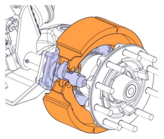
. Install the brake drum as previously recorded on the drum and wheel stud during the removal procedure.
