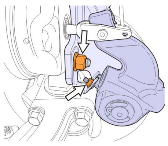
. Remove the snap ring and washers securing the slack adjuster to the brake S-Cam.
