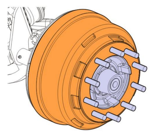
. Install the wheel using the reference marks made on the wheel and the wheel stud during the removal procedure.
