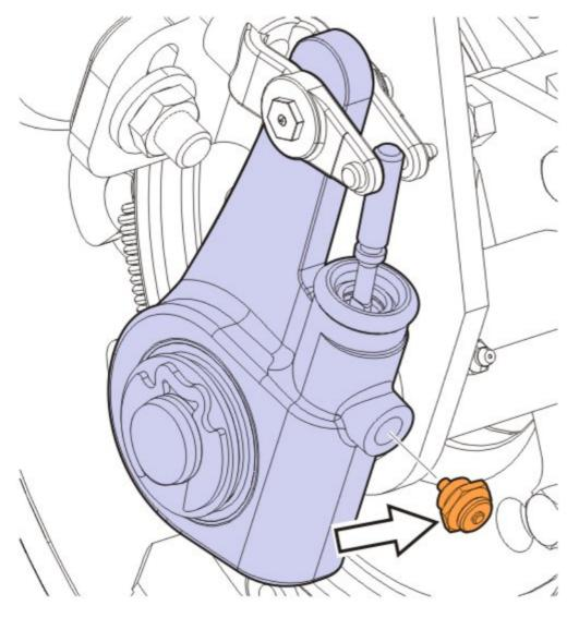
. After brake the adjustment, rotate the wheel and ensure the brake is not dragging or the drum is not out of round.
