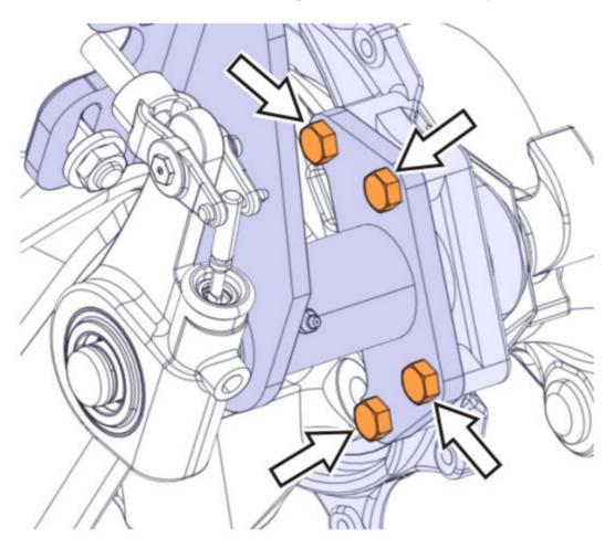
. Remove the brake S-Cam by pulling the S-Cam clear of the cam tube and brake spider.
