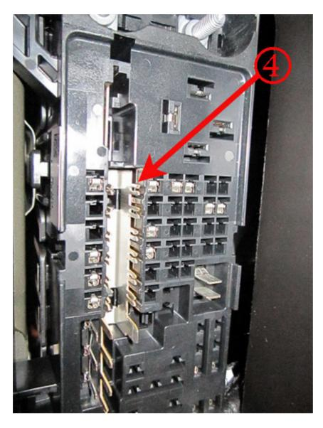
If the loose connection is found to be with the main power buss bar (4) or the plastic fuse block body is deformed, replace the complete Rear Fuse Block with GM Part number 13586872. The new Rear Body Fuse Block will include the main power buss bar and the black plastic body, shown below. All fuses/relays/terminals will need to be transfer over from the old fuse block.
