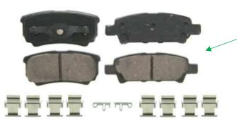
Correct parts should measure: 4.165" - Inners 3.175" - Outers Affected parts should measure: 7.11" - Inners 7.11" - Outers
