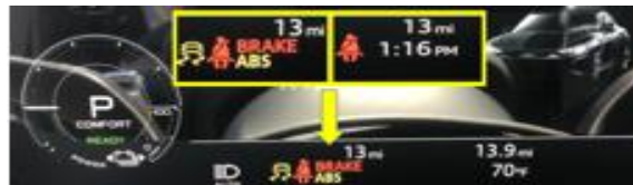
Figure 1. Traction, brake, and ABS lights flash on/off together.
