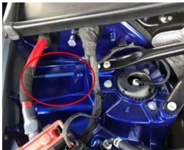
Figure 2. Area with poor finish near the VIN stamping.
